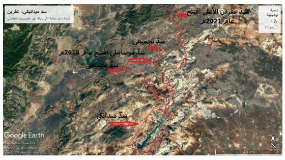
According to a private source, the regular storage volume of Maidanki Dam (190 million cubic meters) is at the level of 335 meters, and the minimum storage volume of (12.5 million cubic meters) is at the level of 298 meters, while the current level is 322 meters, and the minimum level for the work of the dam is 320 meters.
